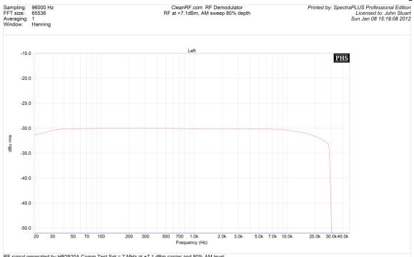
RF signal generated by HP2920A Comm Test Set = 7 MHz at +7.1 dBm carrier and 80% AM level. RF Demodulator BNC output to M-Audio Delta 1010LT soundcard calibrated with Fluke 289 True RMS Meter at 1kHz.
